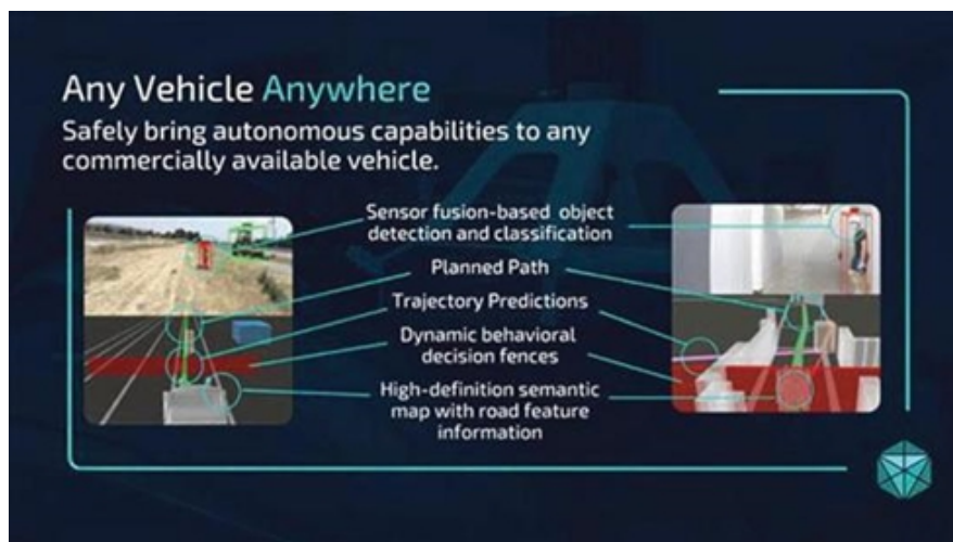
Figure 4: Illustration of DriveMod's ability to utilize key subsystems across multiple environments and vehicle platforms (left: off-road utility vehicle; right: indoor material handling vehicle).
